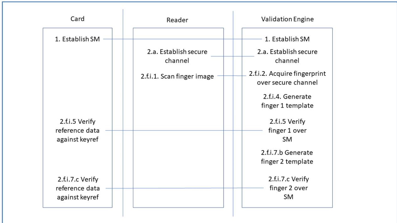
Figure 2 - Secure Channels and checklist command flow
